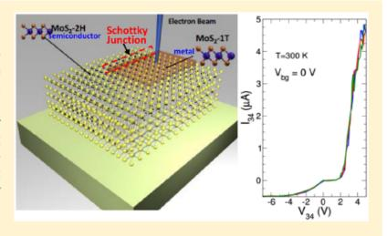
simulation, reveal unique device fingerprint of SB-based field-effect transistors made from atom-thin 1T layers.
